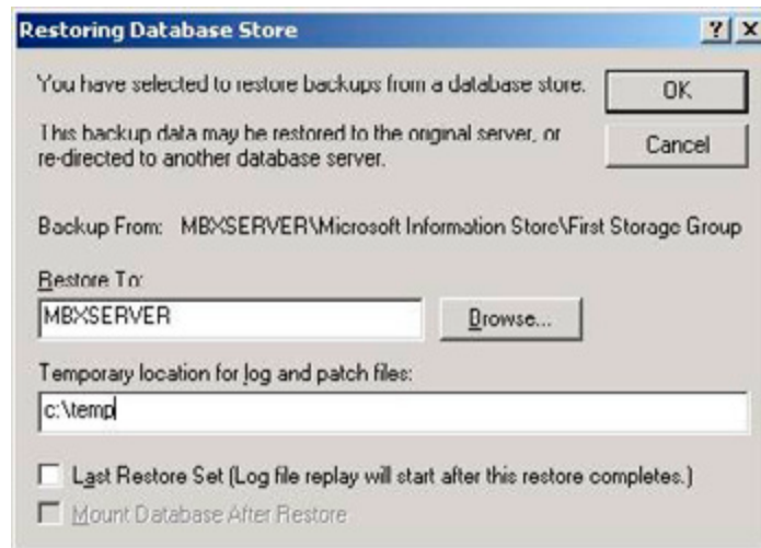
Figure 3. Is this really the last restore set? If so then checkmark the checkbox
